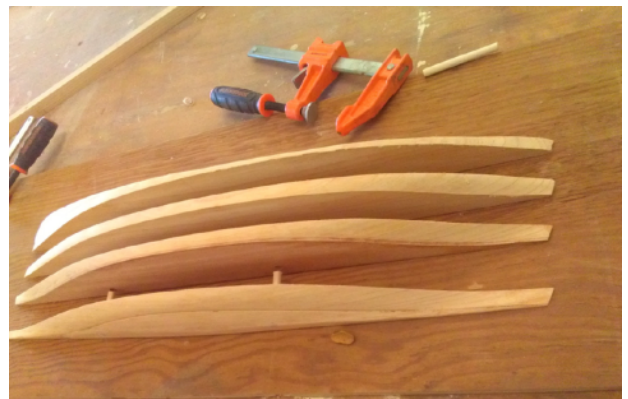
Hull shape achieved, ready for glue up
