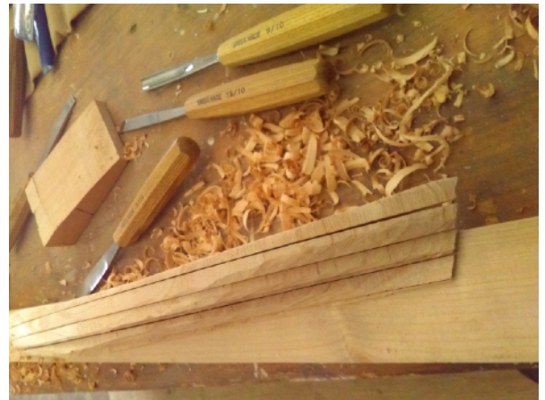
Hull shape revealed by careful carving
